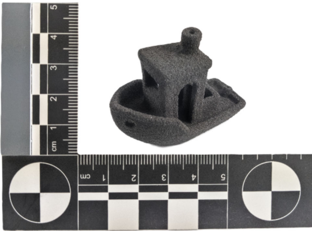
Figure 8. Illustration of a #3DBenchy model printed with sintered bauxite sand.
